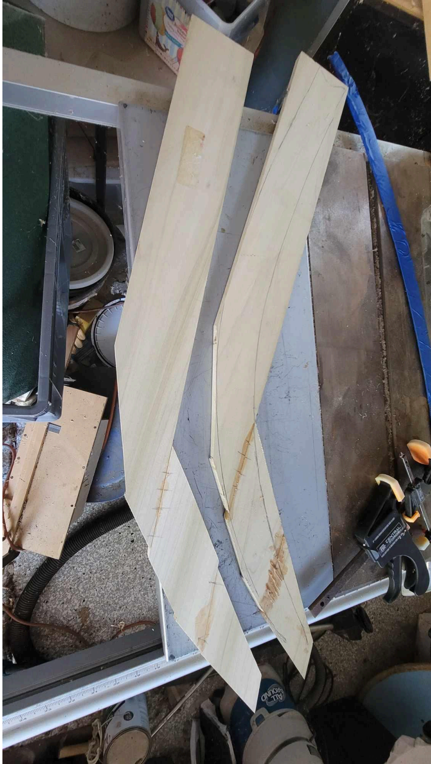
Above: three stages of tracing and joining the wood for a scabbard with a severe curve. In this case the old low-quality scabbard was used as a template. The hash marks on the joints were used to align during glue-up.
