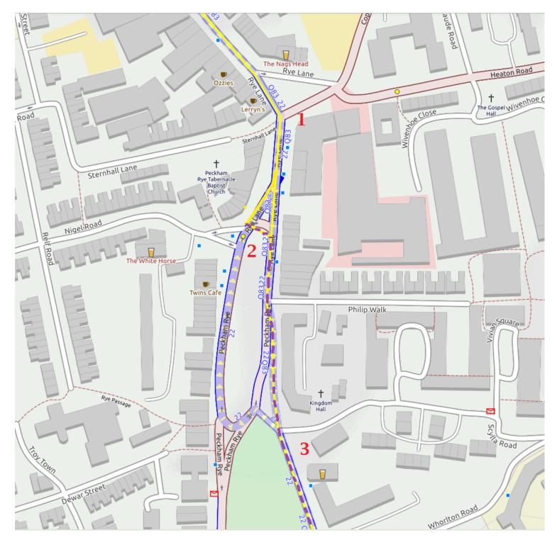
**1** - Cyclists come from Rye Lane to come onto a protected cycleway which goes past Tesco, bypassing the bus stops, before joining a bidirectional track (shown in dashed purple).
