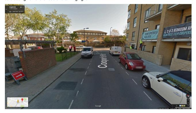
**Solution**: currently Cooper's Rd. (a residential street) is used as a shortcut from the A2. onto Rolls Rd., filtering this shortcut would make this turn a lot less hazardous (given the alternatives available). The removal of parking from the approach of Cooper's Rd onto Rolls Rd. is also an option to improve sight lines.
