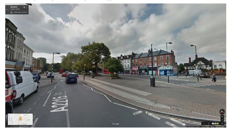
The road needs to be realigned so that much of this dead island space is 'given' to the Tesco side (as it were). There are indications that the island has been *expanded* a few times in the past (clearly seen in the photo above). This way not only do pedestrians have more space to breathe but the cycleway will work much better and cause less conflict. The realignment of this area seems a real possibility.
