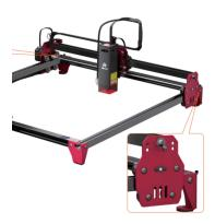
Then we install the shims and screws while tugging on the Y-axis belt by hand or pliers.
