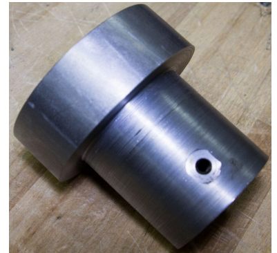
Figure 19. Side View of the Nozzle. The smaller diameter of the nozzle can be seen along with the hole for the pressure sensor.
