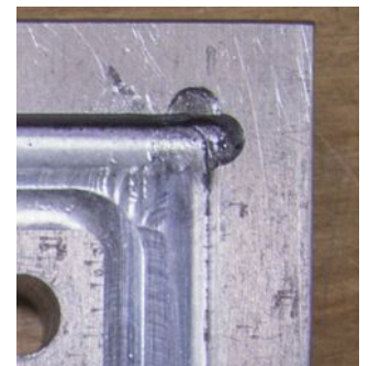
Figure 4. Close-up View of Back Metal Plate. In the top right corner, the CNC machine cut too far causing an unnecessary cut.
