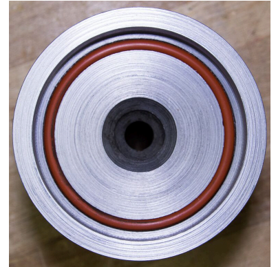
Figure 18. Front View of the Nozzle. Above is a view of the nozzle looking down the throat of the nozzle. The o-ring can be seen along with the counterbored hole
