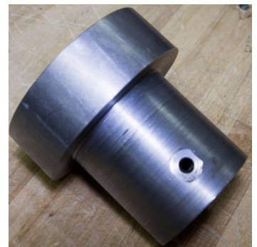
Figure 8. Steel Nozzle. Above is a close up view of the nozzle showing where steel tube was cut down.
