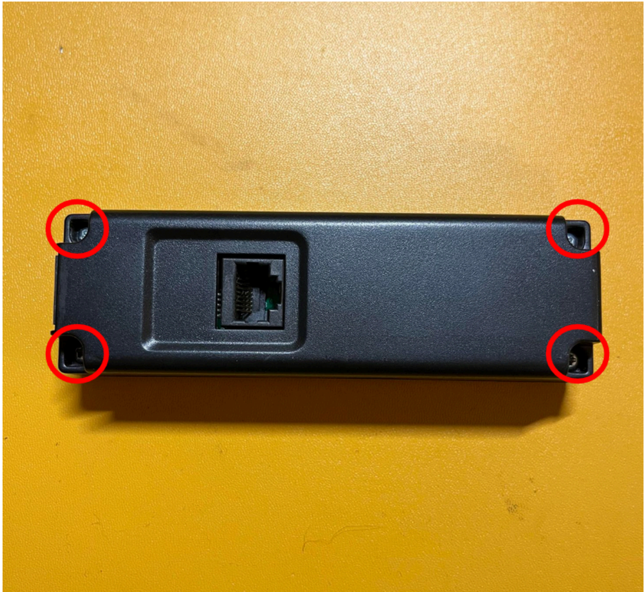
Figure 1. Back of Scangauge II, screws location
