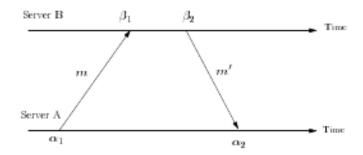
Consider the exchange of messages between two time servers A and B above. Each server has a local clock which he uses to timestamp events, i.e.,  $\alpha_1$ (resp.  $\alpha_2$ ) is the timestamp of sending message m (resp. receiving message m') by server A's clock. Similarly,  $\beta_1$  (resp.  $\beta_2$ ) is the timestamp of receiving message m (resp. sending message m') by server B's clock.
