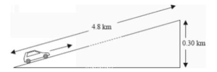
The car moves up the incline at a steady speed of  $16~{\rm m~s^{-1}}$ . During the climb, the average friction force acting on the car is  $5.0~{\rm '10^2~N}$ . The total weight of the car and the driver is  $1.2~{\rm '10^4~N}$ .
