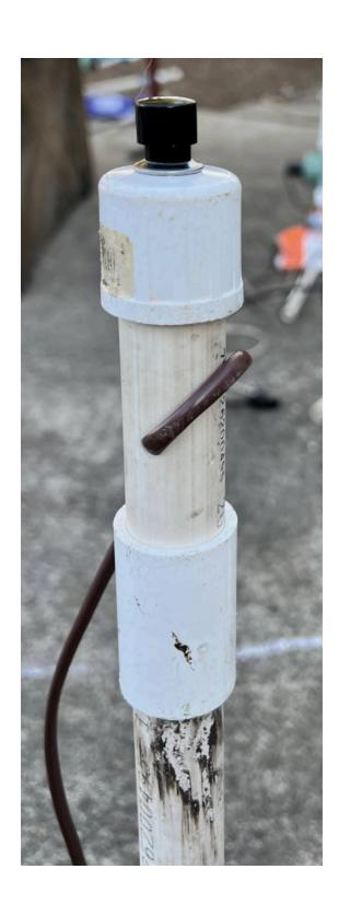
4. Button opens valve and releases air which launches the rocket
