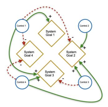
Dynamic system goals can be balanced through feedback (both positive or negative) from embedded controller mechanisms.
