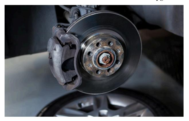
Alt text: Carbon ceramic brake rotor and caliper mounted on a car wheel hub with tire removed for service.
