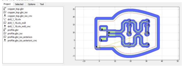
You should now have (at least) two .nc files: one for the traces and one for the outer profile, plus one or more for any drill holes in your board.
