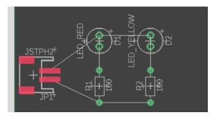
The white lines connecting the components are "airwires". They indicate stuff that has to be connected, but isn't yet.
