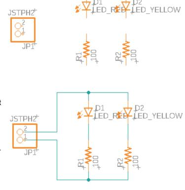
Next, assign values to the resistors with the **Info** tool. Use a resistance of 100 ohms for a red, yellow, or green LED, or 50 ohms for a blue or white one. Of course these are just labels for your convenience, you can put whatever parts into the circuit board you like.
