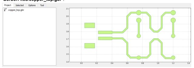
We can see the copper traces we planned out in Fusion. Now, we want to make our CNC mill trace along the outside edges to "isolate" these traces from the rest of copper on the surface of the board. Double-click on copper\_top.gbr. Set the "**Tool dia:**" to the cutting tool diameter, in mm, you intend to use (for instance, 1/64 inch = 0.4 mm).
