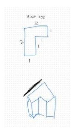
The concept sketch I created resembles a 2x2 block, but with a corner section removed, featuring 1x1 dimensions. Additionally, I incorporated a 2x1 extension to ensure that the block's edge aligned correctly and fits seamlessly between the corners of the other pieces.
