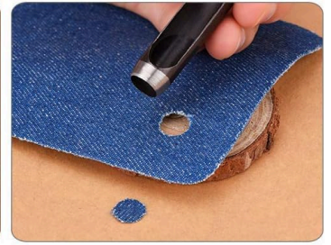
3. Tap around the bottom of the cutter evenly, punch the hole.
