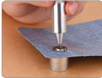
6. Put grommet on the matched mandrel according to the diagram.
