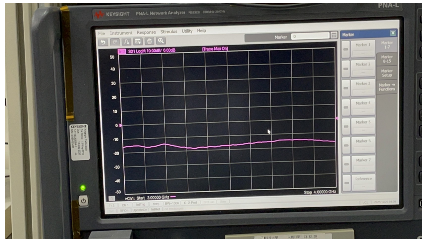
Fig.18. Keysight PNA-L Network Analyzer N52328 used for S parameter measurements
