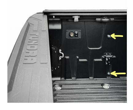
6. You'll then use an oscillating multi tool to cut a precise hole for the power switch and easy access coupling mounting bracket and its associated bolt holes. Use the bracket as a template and mark your cuts carefully. Mount the bracket using the supplied hardware and place the switch and coupling insert in the bed wall. Wire the switch and air compressor coupling according to the ARB factory instructions.
