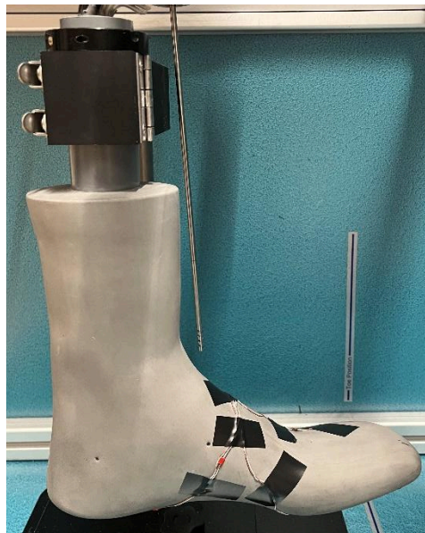
Figure 2: Moulded test foot with sensors
