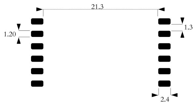
It is recommended that the stencil be 8 mil in thickness to ensure enough solder paste can flow into the castellations.
