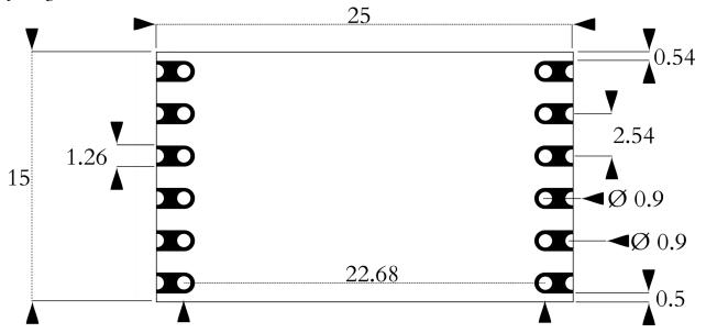
Figure 1. Physical dimensions of the module.
