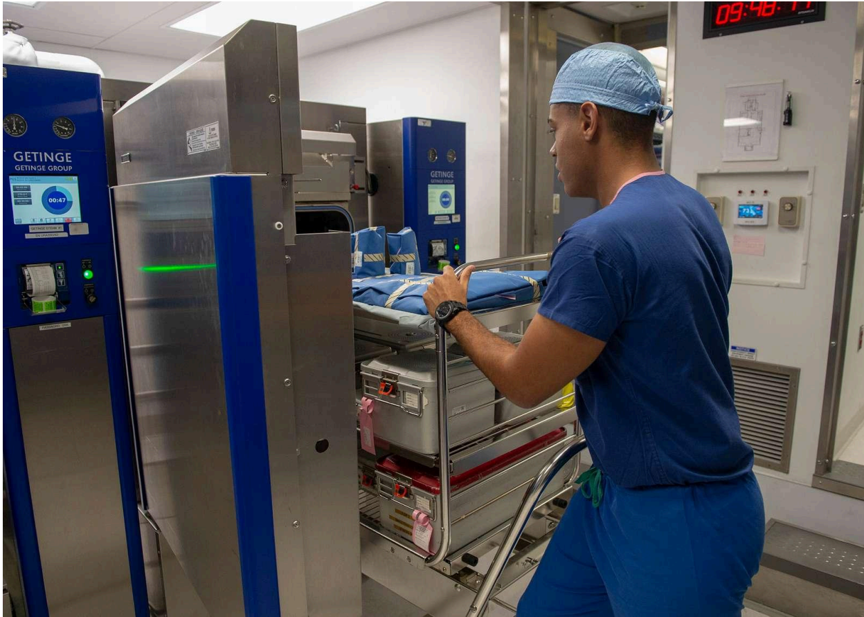
An autoclave uses high-pressurised steam to sterilise equipment. ( Image source )
