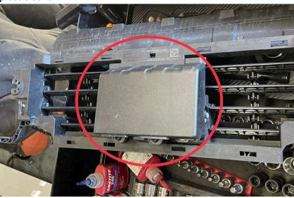
b. Remove 3 bracket bolt and separate from shroud. The disconnect sensor from harness and separate sensor from bracket.
