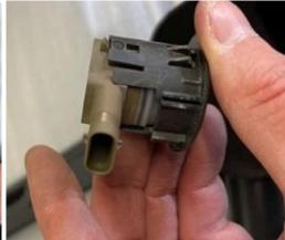
5. Connect wiring harness to sensors. Then proceed to next steps to install the bumper in section 3.
