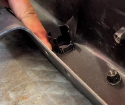
3. Install back plastic sensor trim pieces into new bumper. Take note of the correct orientation for proper fitment, the small tab on the side indexes into the small tab on the bumper.
