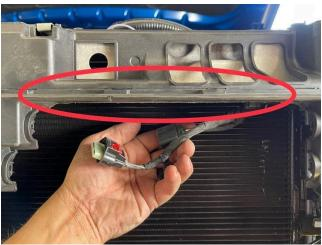
b. Fit the bracket as desired, mark, drill and install with supplied hardware. Then install sensor onto the bracket with supplier hardware & connect to harness.
