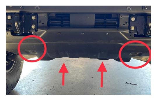
2. Remove the plastic trim panels that cover to expose the bumper attachment bolts. (4 Plastic panel clips each side), pry off with panel tool or pull backwards on each side.
