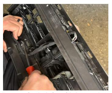
e. Reinstall harness by passing it from by the front of the battery, and exiting by the original harness connector. Reconnecting to factory main harness. Then re-route the remaining harness along radiator and pass sensor connector to into the inner grill section with the removed louvers/ fins.
