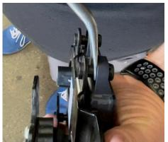
c. Remove 3 gromets from sensor by pushing from front and prying tabs on the back.
