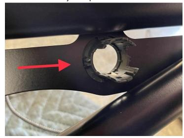
4. Install sensor into plastic trim pieces. Take note, the sensors fit into the black trim pieces in a specific orientation.
