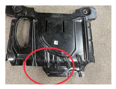
3. 2.7 Engines or vehicles equipped with a transmission cooler will need to trim the bracket as shown below on the driver's side.
