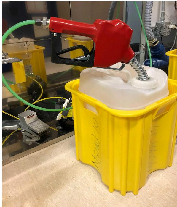
**11.3.3** Locate the pump's foot switch — Press the foot-switch with your foot, and squeeze the pump handle to empty the small front carboy into the larger carboy. If you did not start a new large carboy, keep an eye on the liquid level and make sure you do not overfill the large carboy.
