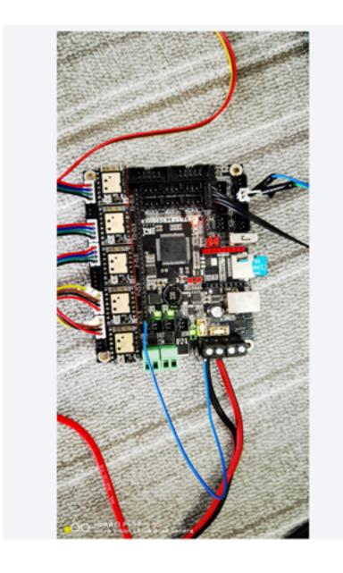
The figure below shows how to use the alternate method of connecting MGND to GND using a jumper wire. Again, note that only two jumpers need to be connected between MGND and GND and not one for each driver.
