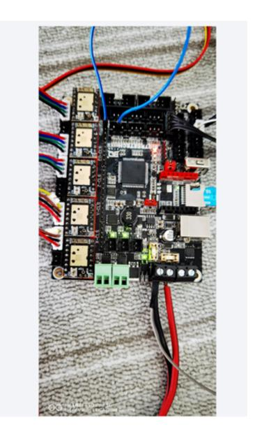
NOTE: The advantage of using either of the above methods is that when you want to use one or more TMC drivers, you can simply apply the hardware jumpers and the firmware modification. If, however, you decide to use a full set of drivers that do not include a TMC then you can simply disconnect the hardware jumpers and re-enable the driver anti reverse feature in the firmware.
