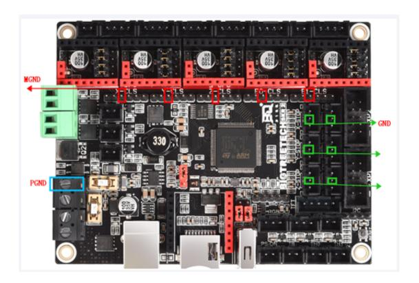
The figure below shows one dupont cable going from MGND to PGND. Note that only two cables need to be used at most. Not a cable for each driver.
