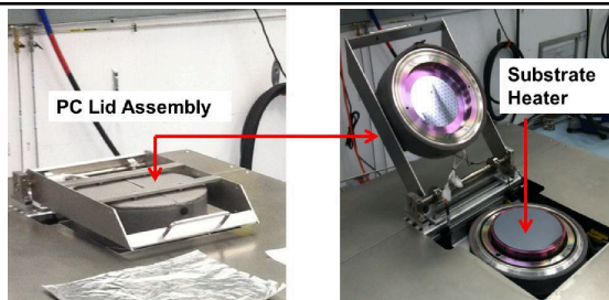
Mechanical stops support PC lid in open position
