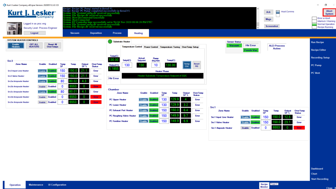
Fig 13: Heating screen. Note the different heating zones, e.g., Chamber, Src 3, etc.
