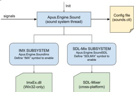
How it works: you call InitSoundSystem() to start the sound system, which works in a separate thread. If you're using the GameApp unit (framework) - it calls the initialization for you. Then it loads the config file (default: sounds.ctl) from the current folder. This file defines all sounds and music. If there is no config file - the sound system won't run and you don't need underlying libraries.
