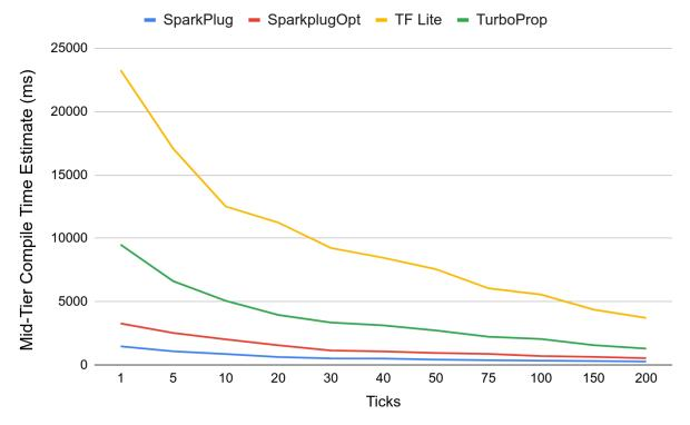
As expected, at aggressive tick-thresholds the amount of time spent in compilation can be very high, particularly TurboFan-Lite which spends 5x more time compiling mid-tier code than executing JavaScript. In general, compared to TurboFan-Lite, TurboProp takes around 1/3rd of the compile time, SparkPlugOpt reduces this to 1/7th and SparkPlug is faster still at 1/16th of the compile time.
