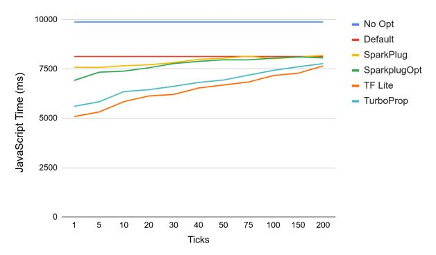
In general the Maps page performs well with optimization. It already gets a 17.7% reduction in JavaScript execution time with TurboFan (No Opt compared to Default). At the most aggressive tick-thresholds, TurboFan-Lite can provide an additional 37.4% reduction, with TurboProp not far off at 31% reduction (both compared to Default). It is clear that most of this benefit is coming from speculative optimization when we compare SparkPlug (6.7% reduction) and SparkPlugOpt (14.9% reduction).
