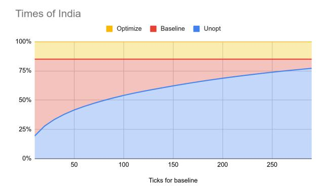
Times of India also spends less time in TurboFan (around 15% of ticks, although we know from experience that in the real-world it is even less due to type feedback updates), with a middle tier, potentially having between 45-55% of execution if tiering-up at between 20-50 profiler ticks.
