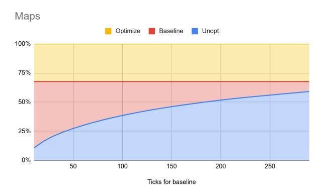
On Google Maps, a good proportion of code is already potentially executable by TurboFan (around 32% of ticks). However there is still scope for executing more code in a middle tier, with around 40-50% of execution being possible in a mid-tier compiler if we would tier-up at between
