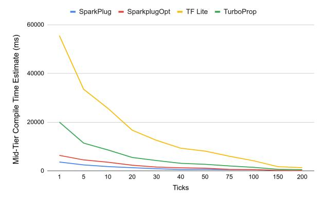
Looking at Amazon the overheads are even larger, with TurboFan-Lite spending more than 7x the time to compile mid-tier code compared to executing JavaScript. The relative time differences between TurboFan-Lite, TurboProp, SparkPlugOpt and SparkPlug are similar.
