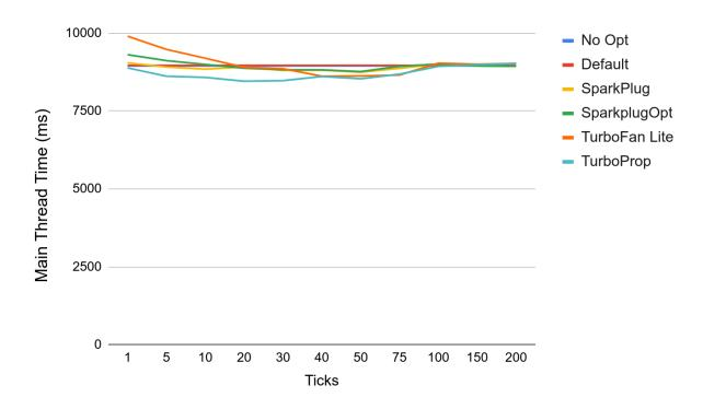
Here TurboProp is on-par with TurboFan-Lite in Maps, and generally better for Amazon. The slope of the graphs also changes showing that, even when looking just at the main thread, being too aggressive tiering up could cause a regression in main-thread time. Overall a tick-threshold of between 30-50 seems the best suited to get the most benefits (similar to what we saw in the <u>Analysis</u> section). For a tick-threshold of 30 ticks, we see the following reductions in main-thread time:
