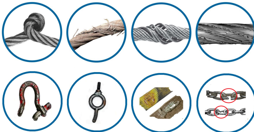
Some Examples of Unsafe Lifting Accessories
