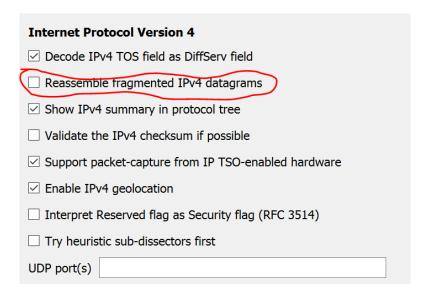
After unchecking the "Reassemble fragmented IPV4 datagrams" box as you can see 10 packets seen in the wireshark but it does not work with tshark command on the linux.
