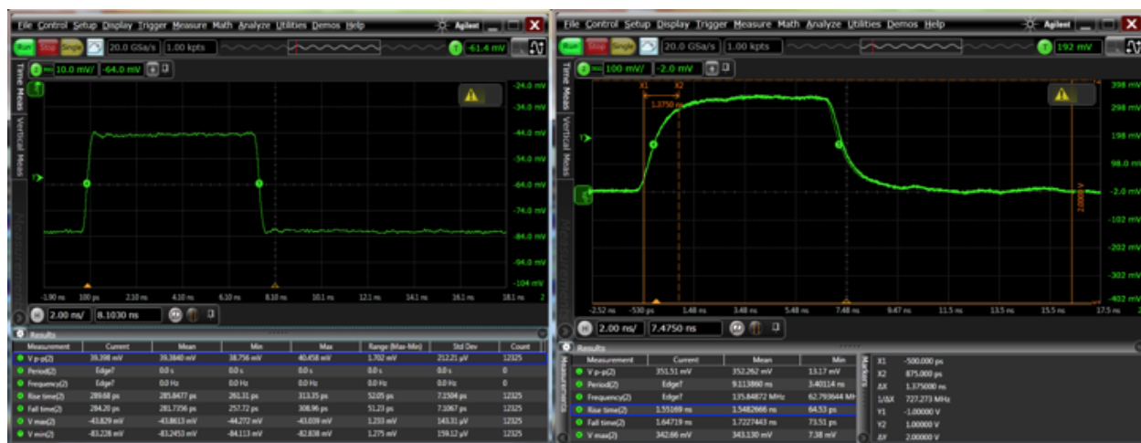
Figure 1.2.4.2. The pulse generated by the ADCMP850 board (left). Resulting signal through the preamp (right). Both were read out by an Agilent GHz scope.
