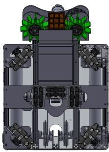
allows us to tuck our pods to the sides of the robot and save a lot of space to build other things like intake and odometry. Getting the spacing between the motor pulley and the wheel pulley right so that the belt had the proper tension took a long time and a lot of trials. We finally got it perfect after the fifth prototype. The pods are
