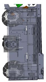
wheels positioned at 45-degree angles.
