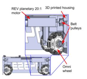
simply screwed into an MDF board that holds the robot together. The large MDF board is where all of our individual assemblies connect together. We also have four side plates to connect the diamond drive pods to each other.
