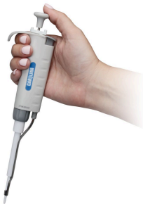
Figure 4. How to hold a pipette: The thumb is on the plunger button used to expel air and suck up liquid. pipette is straight up and down (not horizontal). Tipping the pipette can result in inaccurate measurements, and can allow liquid to contaminate the pipette.
