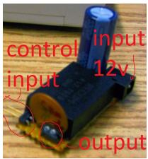
The 2nd prototype pictured at the left was made quickly to put the z axis piezo to work in experiments at Phils lab, this one uses an analog voltage input to control the output voltage, the full scale input for the control signal is 0-4v and for the piezo stack can take a maximum input of 150v therefore the usable range of the control signal is 0-2.1V which corresponds to an output of 95-150V. This is not ideal since we would like it to be able to go down to 0v output.
