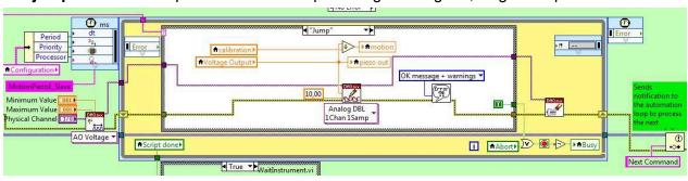
For the **ramp function** I use a For loop in this example. In the second version of the program this will improve.
