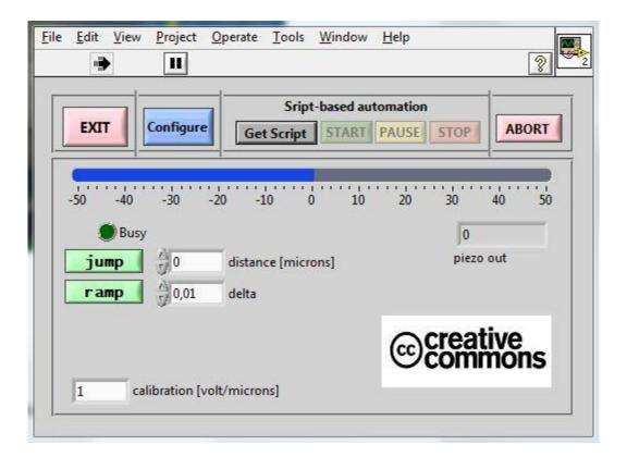
The **jump function** is implemented as a simple voltage analog out, single sample.
