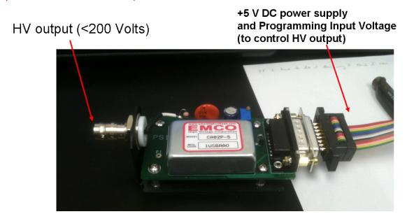
This device takes analog output from a <u>NI PCI-7833R FPGA</u> card and moves the glass needle (See Dilson's project) via the piezotube apparatus (using <u>BPO piezo tubes</u>).
