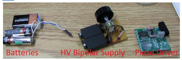
The HV supply circuit uses a dual 5k ohm potentiometer to adjust the output voltage between +/- 95 and 200 V. The recom units are used in this prototype. The batteries were used as there can be problems when using switching power supplies having miss matched switching frequencies and can cause oscillations. The input side of the recom are completely isolated from the output, therefore the **grounds are NOT shared**.
