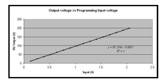
It is powered by +5V DC and has a high voltage BNC (MHV) output. I connect this to the piezotube wires to drive the piezo:
