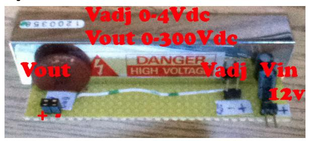
A third prototype was made with the traco units so we have an adjustable output **Vout** of 0 to 150 Volts for the piezo stack (this stack doesn't take negative voltage!), 0 to +/-300 Volts for the cylindrical piezos. **Vadj** should vary from 0 to 2.2 volts for the piezo stack and \*\*\* for the piezo cylinder. **Vin** is 12V.
