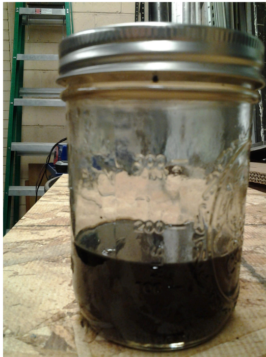
Figure 7. tar and moisture collected by the charcoal filter
