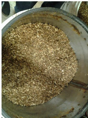
fig2. sawdust (filter media) was in good condition
