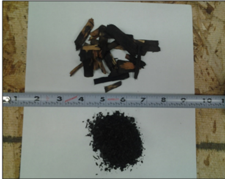
Figure 6. Ashes are compared to the wood chips collected at the bottom of the reactor
