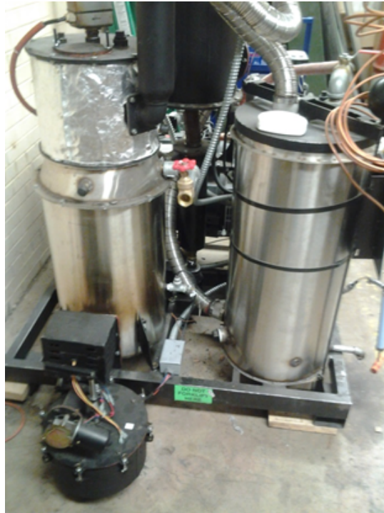
Figure 2. The pilot downdraft gasifier
