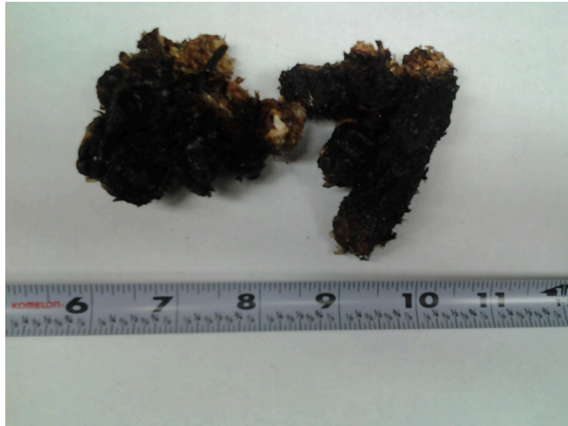
fig7. paper waste-pellet in combustion zone
