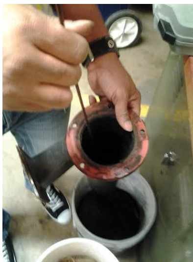
Figure 6. Cleaning the Cyclone
