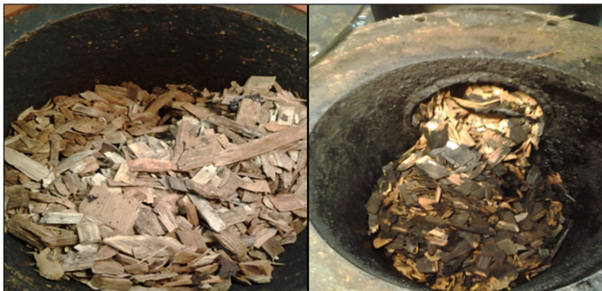
Figure 2. Wood chips at the top of feeder hopper and reactor
