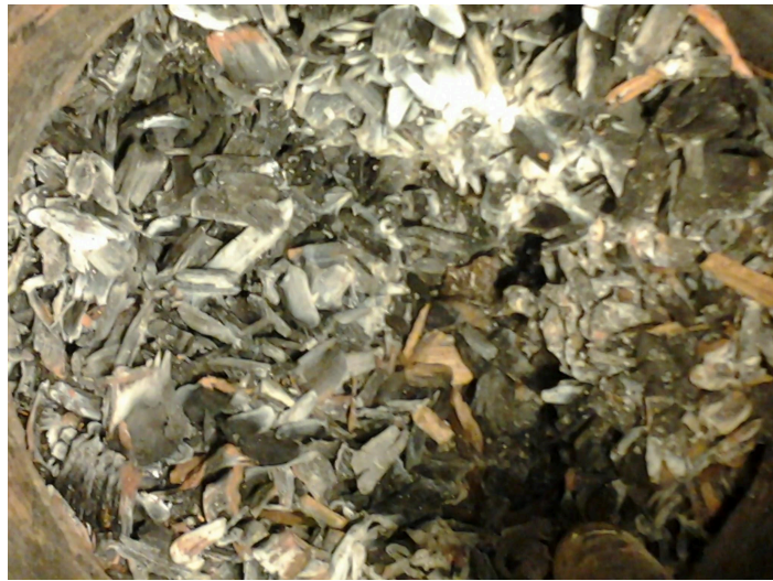
Figure 5. complete combustion at the top of the reduction zone
