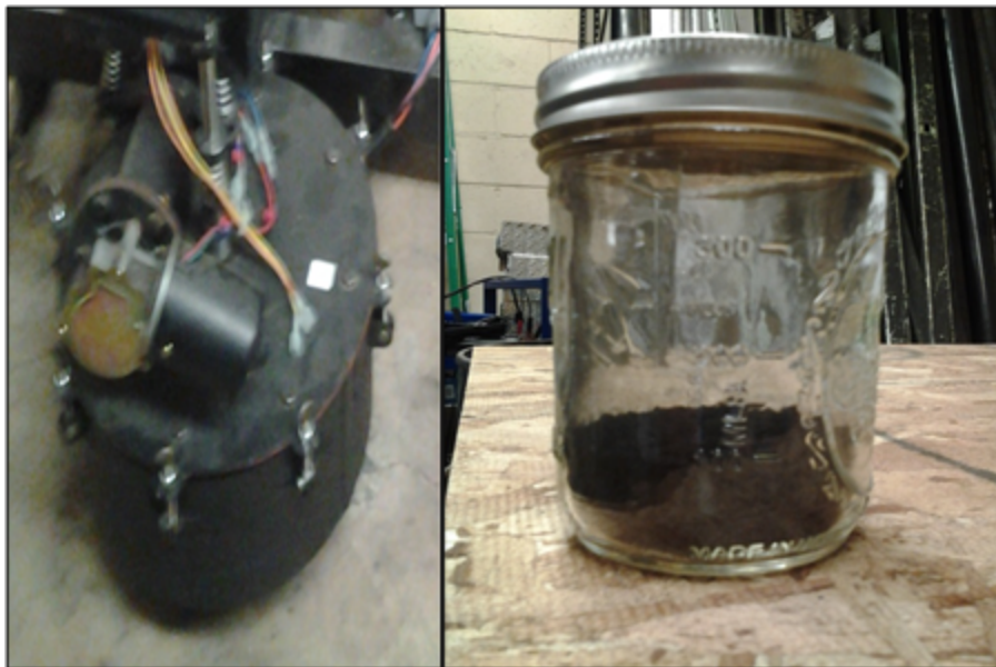
Figure 5. the ash collector and the ash produced during the experiment
