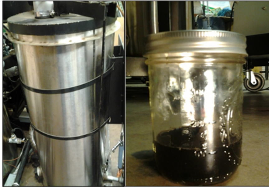
Figure 4. the secondary filter and the collector jar
