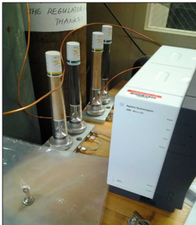
Figure 6. The Gas Chromatograph (GC) with the sample bag
