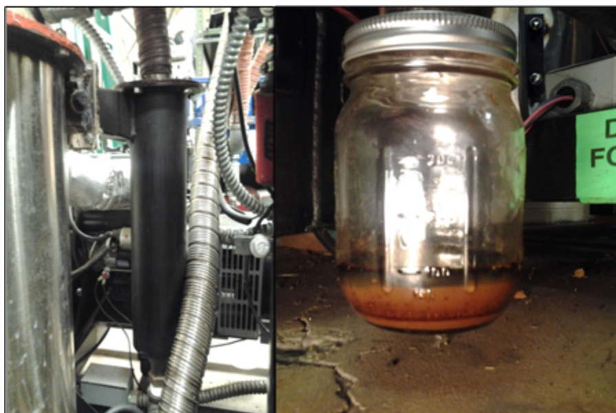
Figure 3. the cyclone and the collector jar
