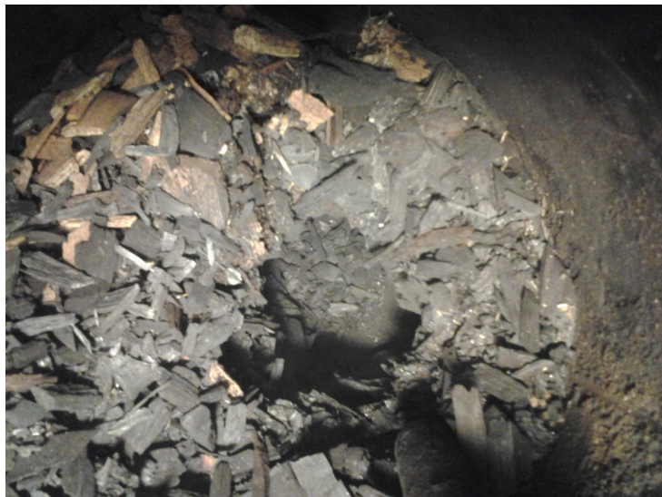
Figure 4. a hole between pyrolysis and combustion zones
