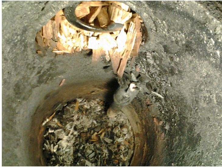
Figure 4. the gap between fuel entrance and top of the reduction zone
