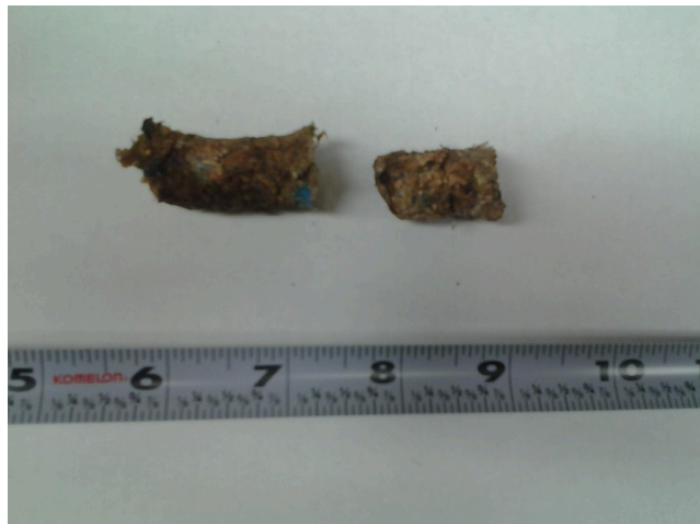
fig6. paper waste-pellet in pyrolysis zone
