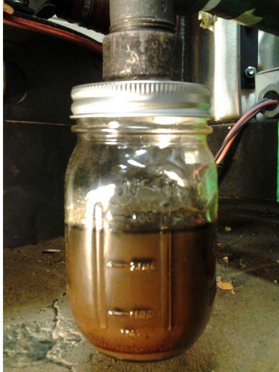
Figure 6. tar and moisture collected by the cyclon
