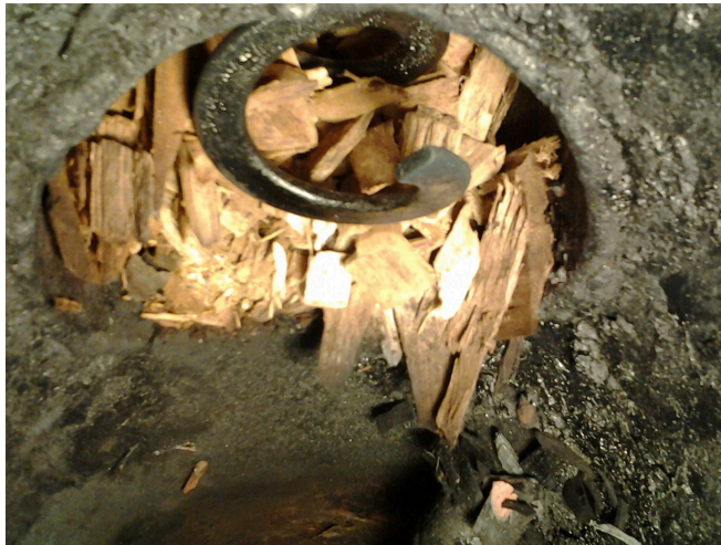
Figure 3. the auger stopped working
