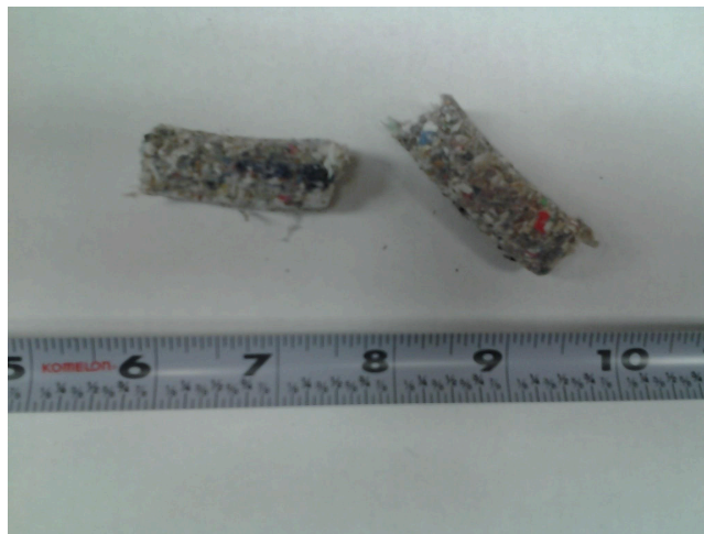
fig5. paper waste-pellet in drying zone
