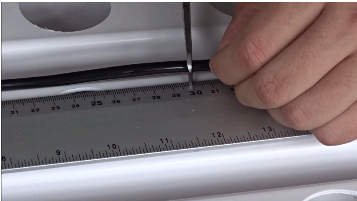
2. Cut to size hose (30cm sections).
