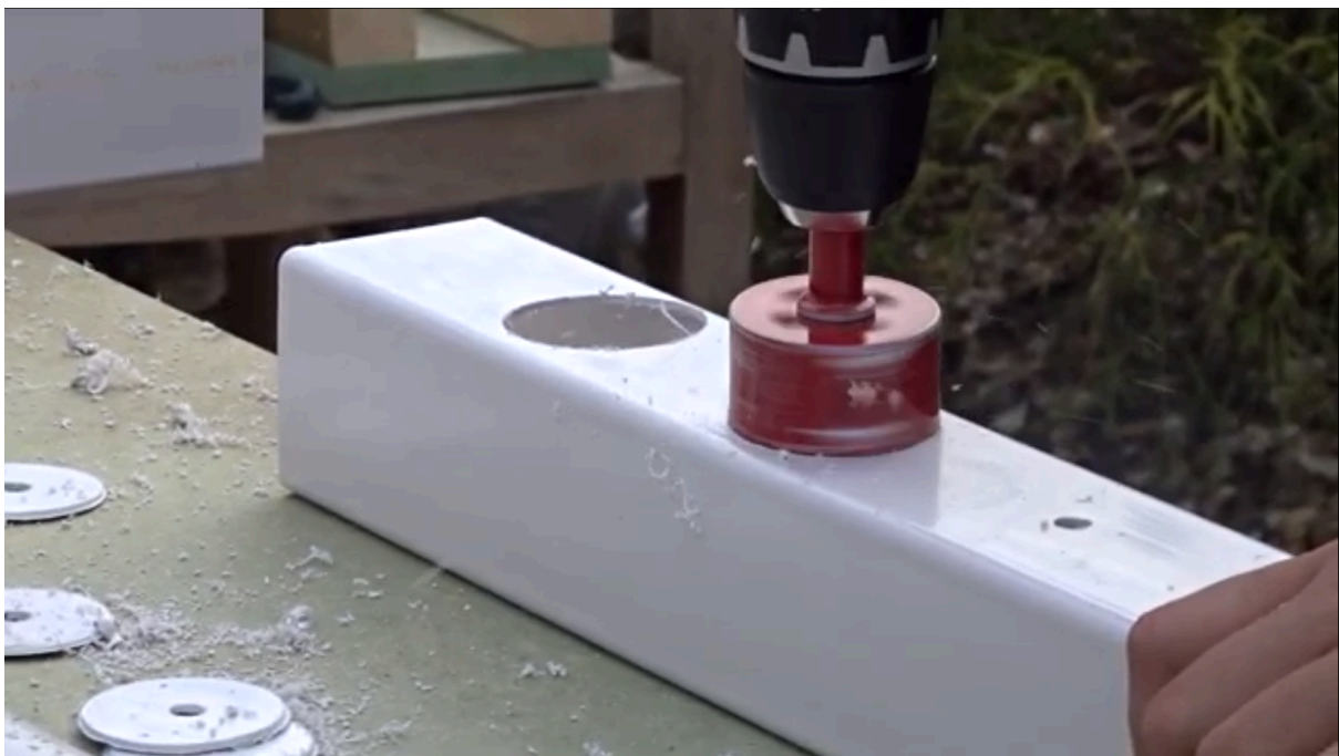
6. Drill plant holes with a hole saw.
