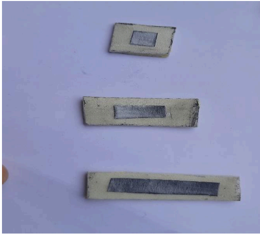
Figure (2)-Graphite on paper sensors placed on the double tape
