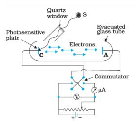
fall on the photosensitive plate C. The transparent quartz window allows ultraviolet radiation to reach the photosensitive plate.
