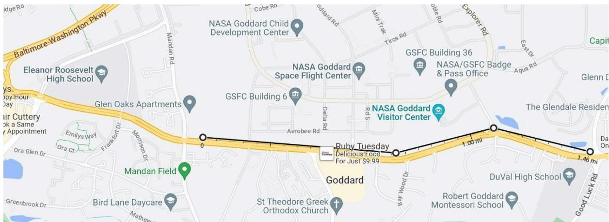
Sector 2 is approximately 1.5 miles long, as shown above. There are two intersections: at Goddard's old "main" gate and at the new main gate at ICESat Road. The trail in this Sector would run entirely on existing pavement, re-purposing existing shoulder space and acceleration/deceleration lanes.
