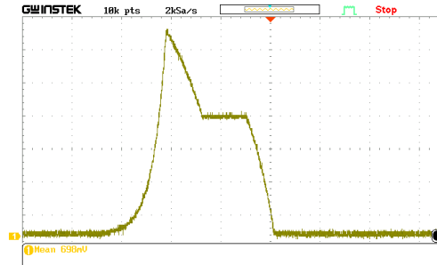
Figure 2. Oscilloscope capture of Exponential envelope curve type.
