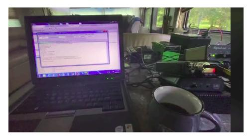
Phil was able to operate Winlink to check and send messages using WD1O's RMS Gateway on 3588 kHz
