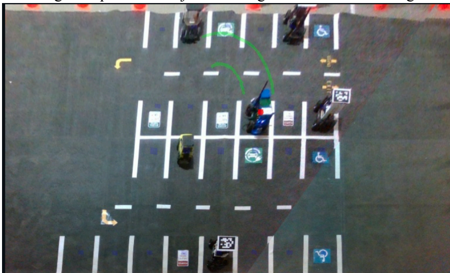
Figure 10: Predicted trajectories using estimated pose and controller input
