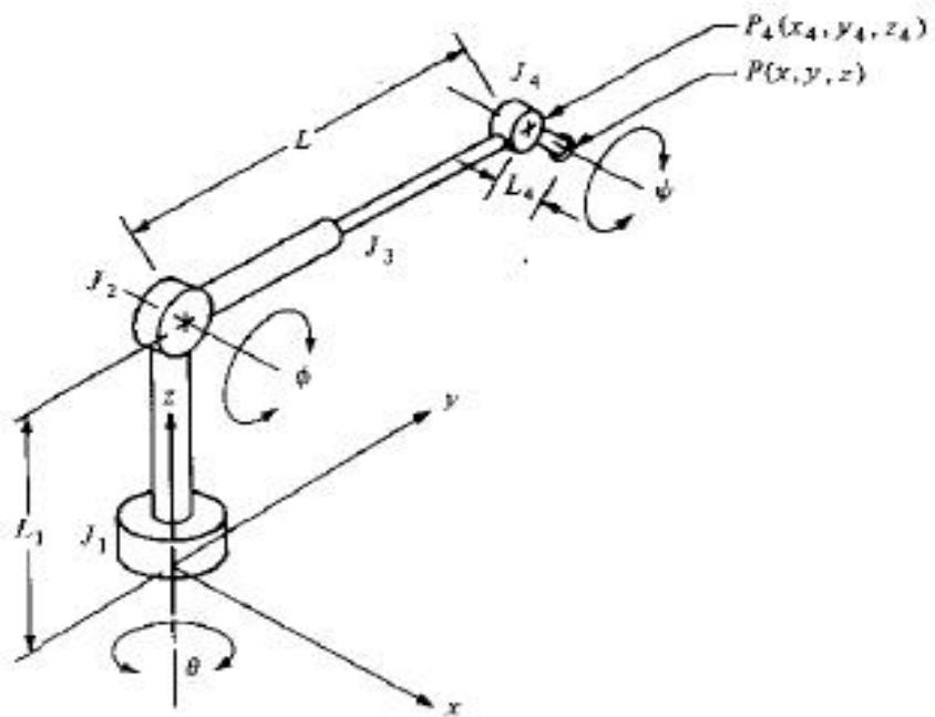
**Forward kinematics:** The position of the end of the wrist, P, defined in the world coordinate system for the robot, is given by
