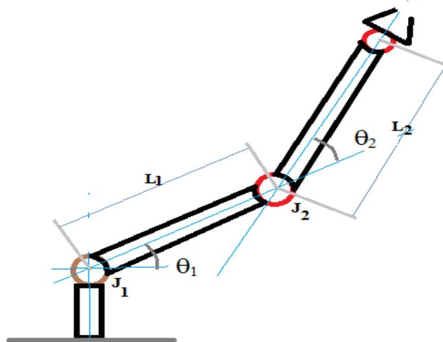
We can determine the position of the end of the arm in world space by defining a vector for link 1 and another for link 2.
