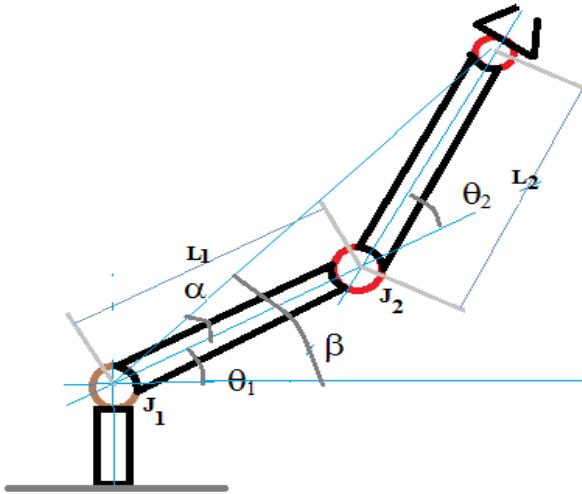
We can find the angles  $\theta_1$  and  $\theta_2$  by using trigonometric identities
