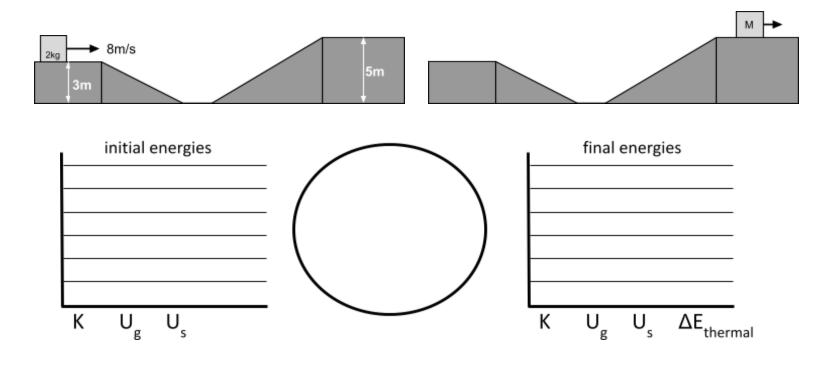
12. A block of wood of mass M=2kg is initially moving 8m/s on a horizontal surface. The box slides down and then up a ramp, and is finally moving along a higher horizontal surface. There's NO friction between any surfaces. Find the speed when it reaches the top of the 5m tall ramp. (System: block only)
