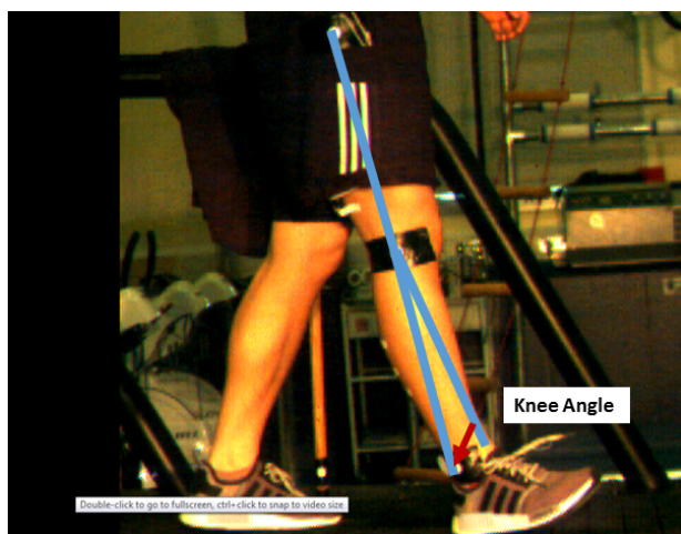
Figure 3: Anatomical land marks for EMG and 2-D-kinematic measures. Snapshot of video image showing the marker location and the knee angle (determined as the angle subtended by the long-axes of the distal relative to the proximal segment) captured during treadmill walking
