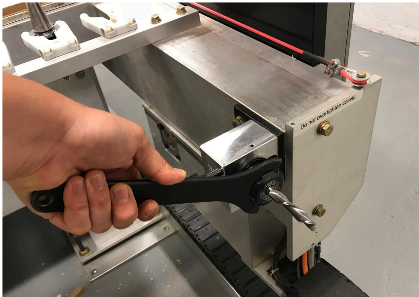
Fig. 5: Using holder for tool cone at the back of the machine and collet wrench to tighten the collet around a bit.
