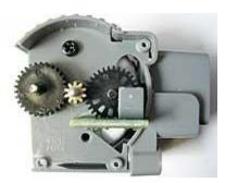
A wheel shaft encoder sensor detects precisely how many times a motor shaft turns by having an encoder sensor monitored as the wheel shaft turns. It has 12 slits in the encoder, and the motor to encoder gear reduction is 10:32, so for each turn of the wheel hub, the encoders turn 48\*10/32=15 turns. Thus, the optical detectors sees 15\*12=180 slits. Using both sides of these slits gives 360 ticks per turn resolution or 1 degree resolution.
