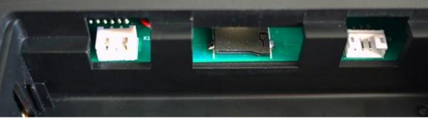
The back of the radio shows the JR-compatible module slot, along with a JR-style jack trainer port, USB connector and earphone jack. The battery bay houses a microSD card slot, a serial port and of course the battery connection.
