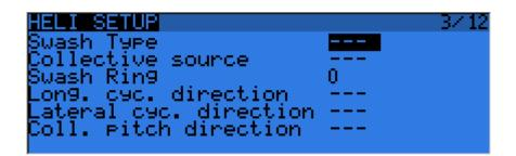
The inputs of this mixer are the Ail and Ele sticks, plus the virtual channel selected in "Collective source". This channel would see entries added on the MIXER page for one or more pitch curves.
