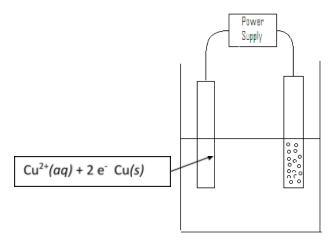
An external direct-current power supply is connected to two platinum electrodes immersed in a beaker containing 1.0 M CuSO<sub>4</sub> (aq) at 25°C, as shown in the diagram above. As the cell operates, copper metal is deposited onto one electrode and  $O_2$  (g) is produced at the other electrode. The two half-reactions for the overall reaction that occurs in the cell are shown in the table below.
