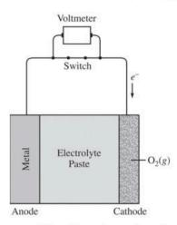
Metal-air cells are a relatively new type of portable energy source consisting of a metal anode, an alkaline electrolyte paste that contains water, and a porous cathode membrane that lets in oxygen from the air. A schematic of the cell is shown above. Reduction potentials for the cathode and three possible metal anodes are given in the table below.
