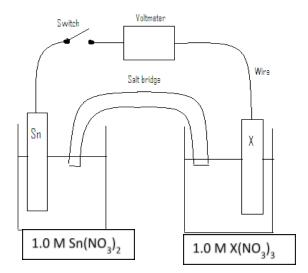
6. An electrochemical cell is constructed with an open switch, as shown in the diagram above. A strip of Sn and a strip of an unknown metal, X, are used as electrodes. When the switch is closed, the mass of the Sn electrode increases. The half-reactions are shown below:
