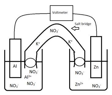
The diagram below shows a galvanic cell based on the reaction. Assume the temperature is 25°C.
