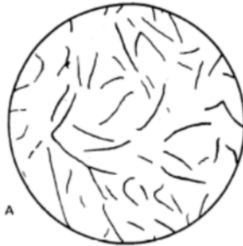
Figure 9: The preferred graphite flake structures for gray cast iron.
