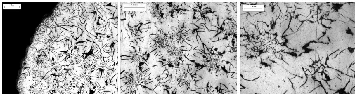
Figure 5: Images of polished and etched sample. (a) shows the inside edge at 100x magnification, (b) show the inside edge at 200x magnification, (c) show the inside edge at 500x magnification.
