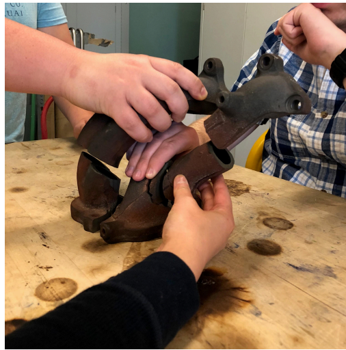
Figure 1: Configuration of how the exhaust manifold should look when all the unattached pieces are reconnected.
