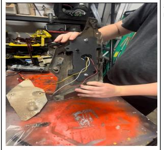
Screw the new light into the bracket, and reinstall the light bracket onto the machine.
