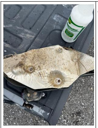
Remove the 4 screws holding the heat shield on .
