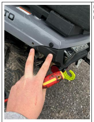
Remove the push pins holding the light on , there are 4 push pins. Then disconnect the plug that goes to the light .
