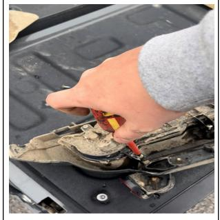
Remove the screws holding the light to the main bracket .
