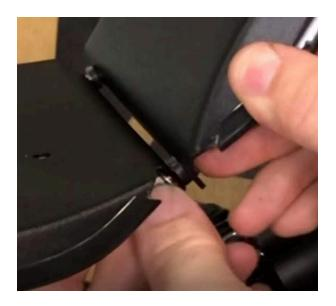
Install seat back to seat tube using the seat back connecter (**first image below**) and skewer. Start with second set of holes. Push skewer through and loosely install skewer nut.
