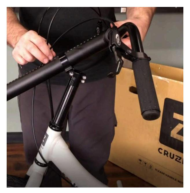
Install the handlebar clamps making sure there is an even gap on the top and the bottom bolts. If one side is tightened all the way down, the clamps can be stressed and break. Make sure there is an even gap as you snug the bolts (**first image below**).
