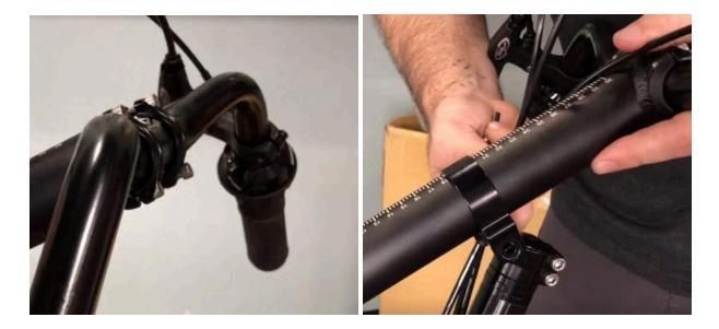
**Note:** if one of your cables ends up on the wrong side of the boom it can be easily disconnected and routed on the correct side of the boom. In the **first image below** the cable ended up on the wrong side of the boom when we installed the handlebar.
