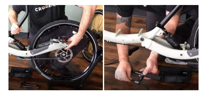
If you have trouble getting the rotor on the wheel between the brake pads, make sure the brake cables are loose at the lever (**second image above**). Sometimes they can get lodged against the stops during packaging which can make getting the rotor between the calipers challenging.
