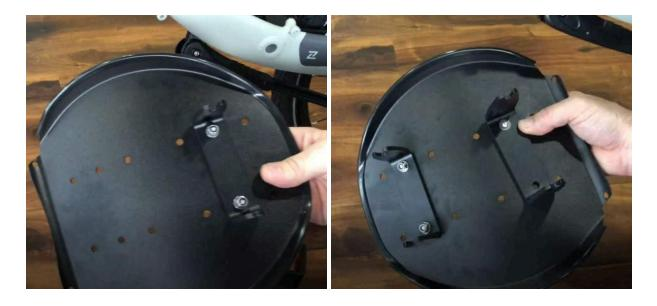
Create a 10 mm nut driver from the Cruzbike Tool Kit. Using the 10 mm nut driver and the 4 mm allen wrench tighten only front bracket bolts. **Leave back bolts very loose.**
