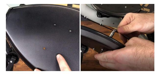
Attach the seat back to the seat pan using (2) 6mm bolts, rubber washers, M6 metal washers and M6 nylock nuts.
