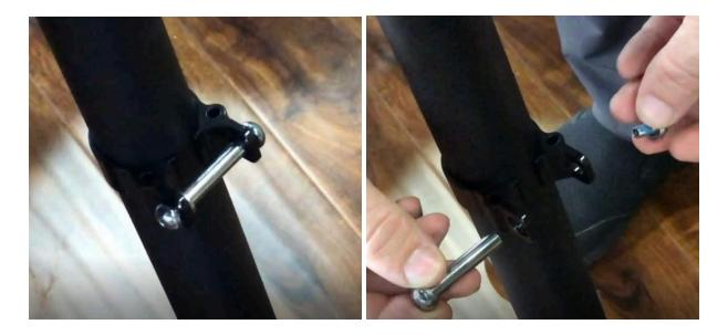
Pivot front end up (**first image below**). If it is difficult to pivot up you may have to loosen the 4mm bolts that hold the boom onto the bottom bracket.
