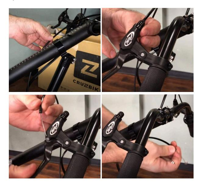
Use (2) 5 mm allen wrenches to snug down the pivot clamp (first image below).
