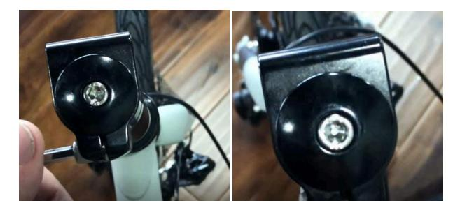
Tighten the top bolt cap one turn. Tighten the side bolts to secure the pivot clamp.
