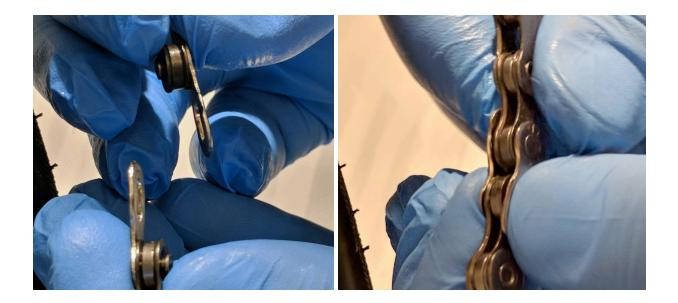
If quick link does not settle into position when pulled (**first image below**) you can place the quick link into the top part of the chain path between the cassette and the front chain ring by very carefully turning the cranks backwards, then push hard on the pedal to close the quick link and lock it into place (**second image below**).
