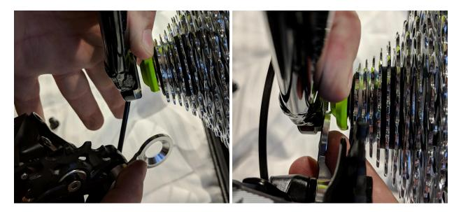
Push the skewer all the way through and tighten the nut (**first image below**). Then, loosen the skewer nut just a little to allow the front end to pivot to finish the assembly of chain and slider.
