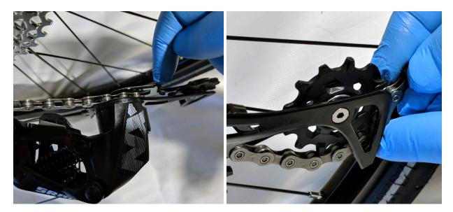
Use the quick link to connect the two ends of the chain together. Inserting the pins into each Use the quick link to connect the two ends of the chain together by inserting the pins into each other. Pull the chain apart to lock it into place. Release the derailleur into its working position by pulling up on the jockey wheel to release pressure and pushing the lock/unlock button.
