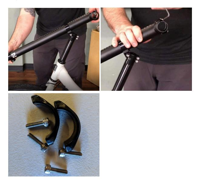
Note the orientation of the cables and rotate the handlebar around to get the cables in the right position. Position the handlebars so that hand grips are vertical (**image below**).
