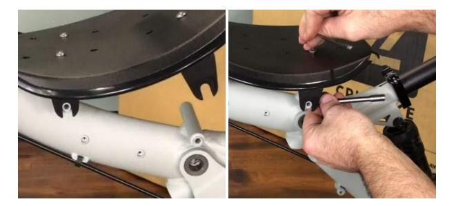
Install the skewers that hold the seat pan to the frame. For consistency, put the lever sides on the brake side, since that's where all the other levers are (**image below**).
