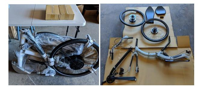
Set the wheels aside and lay the bike frame on a soft surface with the rider's left side up. The brakes, brake tabs and cables will be facing up. Inside and between the padding you will find the seat back and seat base. The front boom and slider and chainstay and crank assembly are separate from the main frame of the bike. The handlebars and shifters are pre-cabled.
