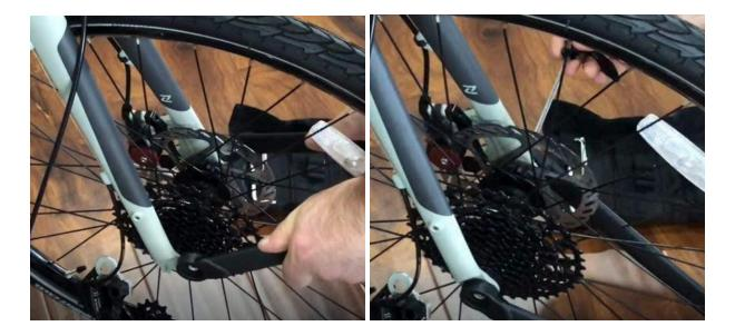
Slide the derailleur between the chainstay and fork. The flat side faces out against the chainstay and the cone side faces against the fork. It only fits snugly and allows the passage of the skewer one way (**images below**). Make sure the derailleur is in the notch on the chainstay.
