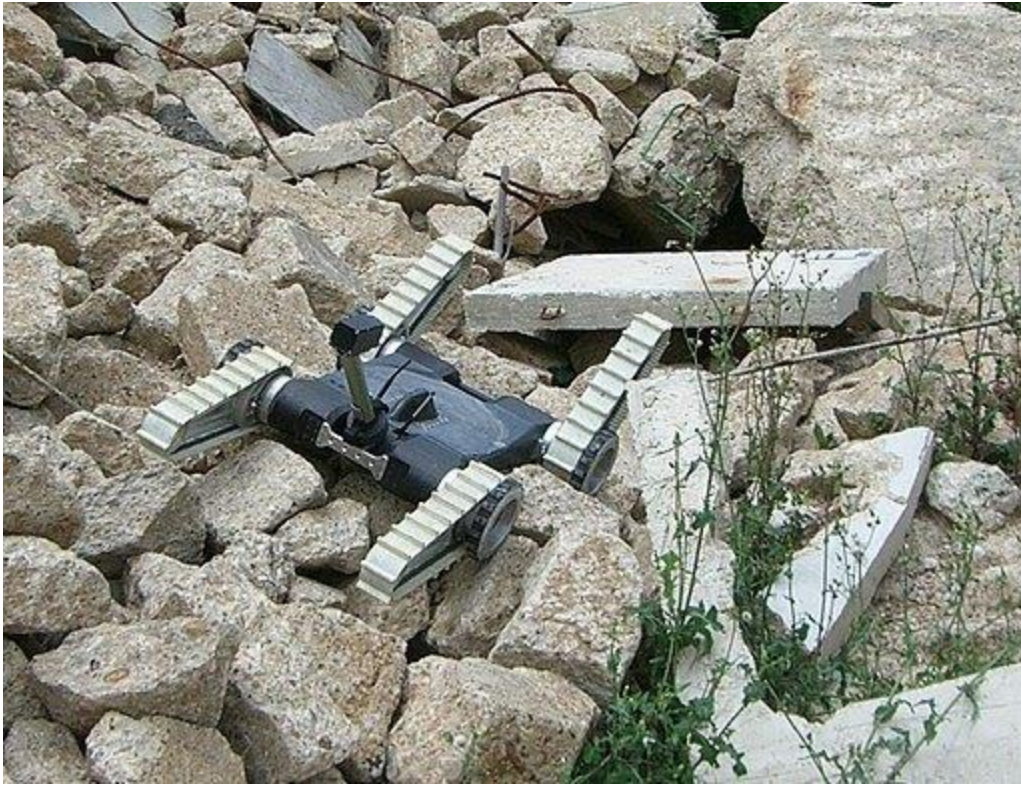
An urban search and rescue robot moves across a rubble pile Photo: NIST [Public domain in the United States]
