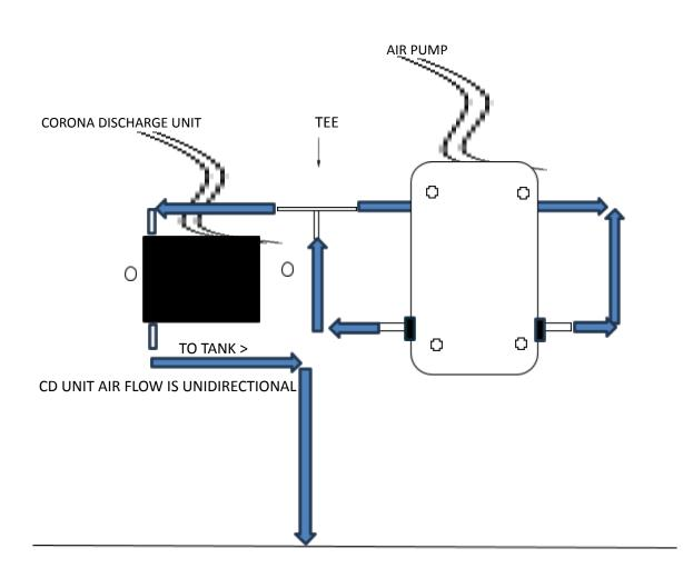
IT IS CRITICAL TO MAKE SURE YOUR TUBING (ON THE OUTPUT SIDE OF CD UNIT IS CONNECTED FREE OF LEAKS! WE RECOMMEND A PRESSURE TEST OF 10 PSI BE APPLIED TO THE HOSES TO ASSURE THERE ARE NO ZONE LEAKS.
